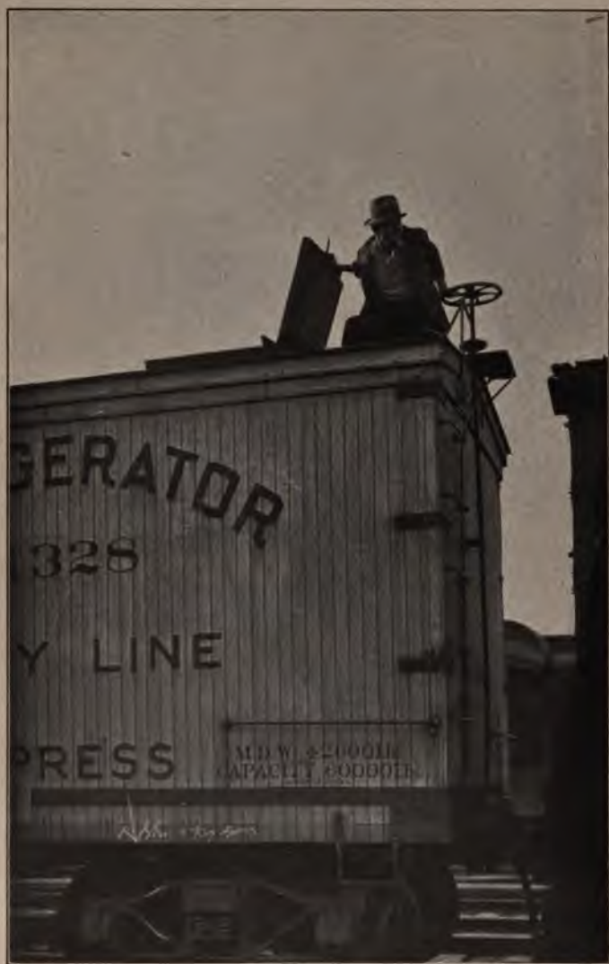
We entered them through hatchways in the top of the car.
